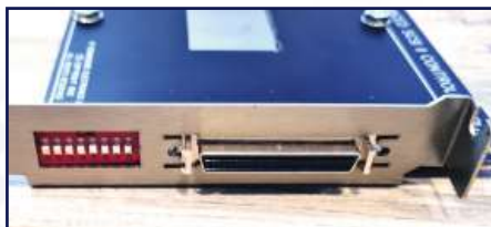
LEFT: DIP switches and external SCSI-2 connector. RIGHT: ReA4091 board fitted, note the connectors for the disk activity status LEDs on the Amiga's front panel.
