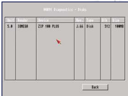
LEFT & ABOVE: Holding the right mouse button at power on provides a useful A4091 startup menu.
