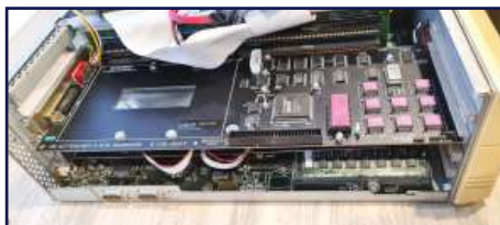
LEFT: DIP switches and external SCSI-2 connector. RIGHT: ReA4091 board fitted, note the connectors for the disk activity status LEDs on the Amiga's front panel.
